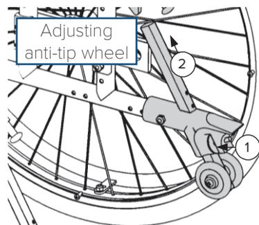
To mount kerbs, lift the anti-tip wheels fully and approach the kerb head-on. Then the attendant uses the stepper tube to raise the front castors, and lowers the front castors on the raised kerb. Finally the attendant should push the wheelchair forward, lifting it up slightly to mount the kerb if required.
