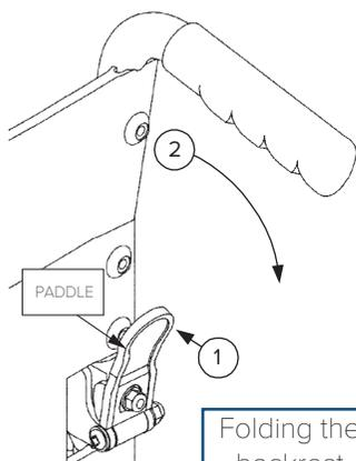
To fold the backrest, push the black paddle towards the back post with your thumb (1) whilst pulling the handle down (2) as shown in the [folding the backrest](#) image. Repeat this operation for the other handle.
