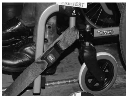
Fitting the front restraint
