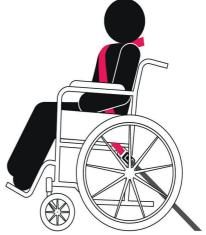
Note: The wheelchair must be secured to the vehicle using a 4-point Tie-down system (not shown on image above).
