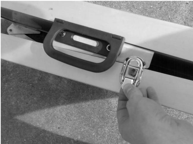
Undo the latch by the handle (as shown on the photo) and unfold the ramps.
