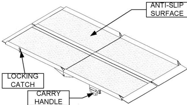
The SMART RAMPs can be used either as a portable or fixed access ramp. The ramps are suitable for a single PMV with user. PMVs (Personal Mobility Vehicle) are wheelchairs, powered wheelchairs and scooters. The ramps can be used to obtain access to motor vehicles, buildings, etc.
